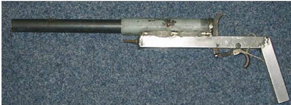
Figure 6 Homemade shotgun made of metal pipe and pieces. Note the simple trigger mechanism.
