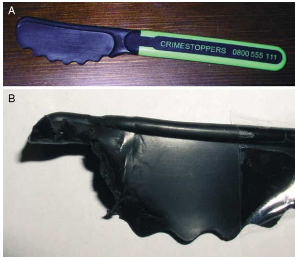
Figure 4 (A) Rubberized knife (blade is flexible and will not cut skin). (B) Close-up of rubberized knife blade after chewing.
