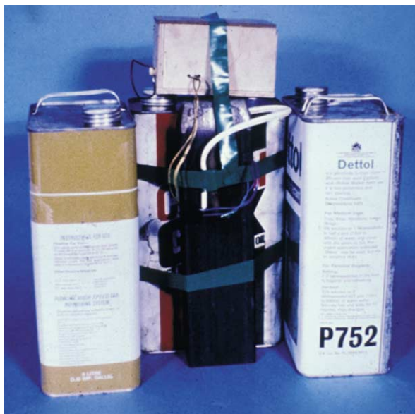
Figure 26 Firebomb. The explosive device is attached to metal containers filled with flammable liquid and designed to rupture on detonation of the device.
