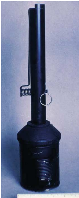
Figure 27 Drogue bomb. Homemade drogue bomb using metal food can. These devices were intended to be dropped or thrown onto passing military vehicles.
