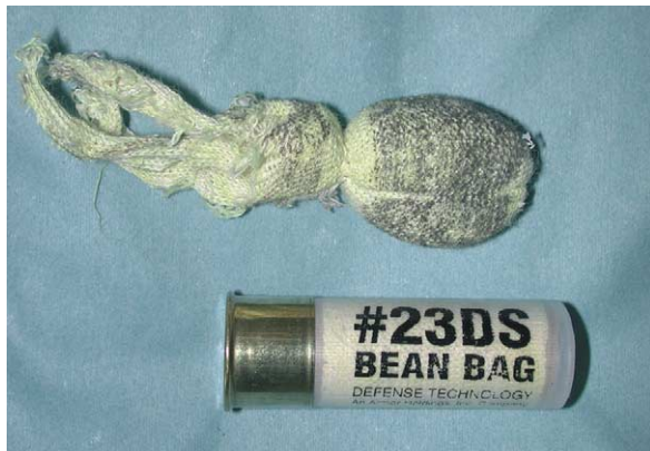
Figure 11 This “sock” round is a less lethal kinetic device, fired from a 12-gauge shotgun. The round, designed to incapacitate a suspect through pain compliance, is capable of inflicting serious injury to internal organs.
