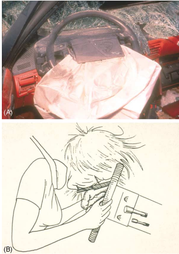
Figure 16 Module covers that split in an asymmetrical manner are more likely to impact facial structures because of a longer arc on opening. This Ford module cover extends 5 1/2 in (14 cm) from the steering wheel hub.
