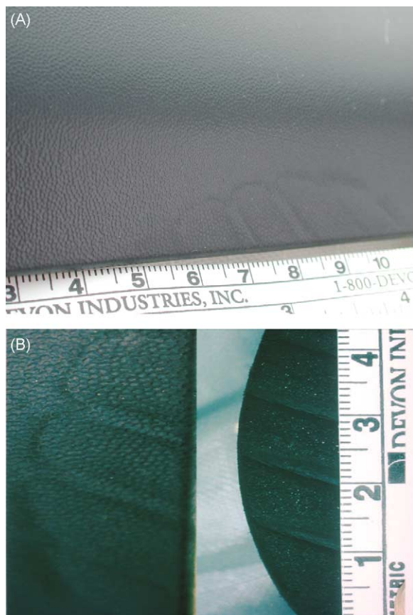
Figure 34 Pattern of the imprint on the module cover matched the sole of the passenger’s shoe.
