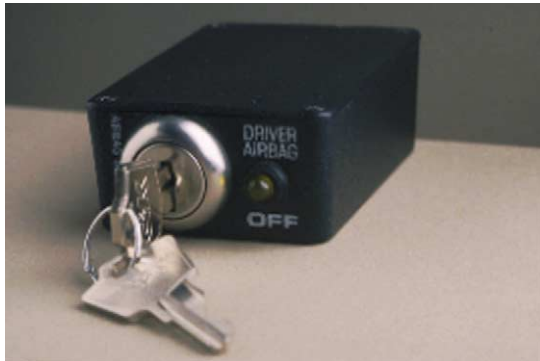
Figure 20 An airbag cutoff switch should be considered for occupants who cannot sit at least 12 in (30cm) from the airbag module ( www.airbagonoff.com ).
