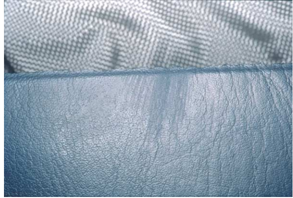
Figure 30 Fabric imprint on module cover is evidence of module cover impact with the patient's forearm.
