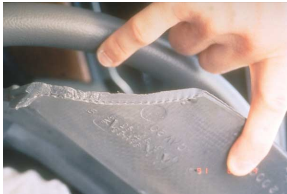
Figure 17 The tearing of this thick module cover occurred when the cover impacted the left side of the face of the woman in Figure 14 . Reproduced with permission Smock WS. Accident Investigation: Airbag-related Injuries and Deaths. In: Encyclopedia of Forensic Sciences . Edited by Jan A Siegel, Pekka J Saukko, Geoffery C Knapfer. Academic Press: London. © 2000 with permission from Elsevier.
