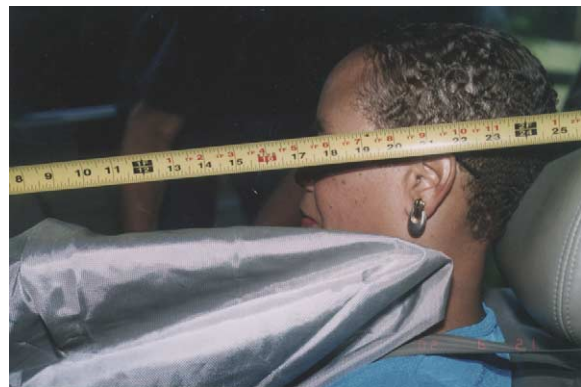
Figure 3 Untethered airbags can extend well into the restrained occupant’s space. This airbag from a Nissan Maxima extended 21 in (53 cm) rearward and was responsible for this patient’s total loss of vision from a ruptured globe.
