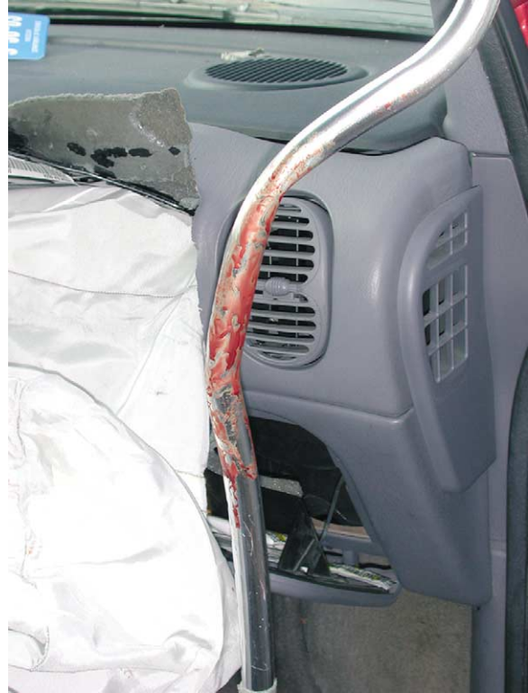
Figure 11 Any objects, like this walking cane, caught in the path of the deploying airbag, can be propelled into the face and eyes of the passenger (Figure 7).
