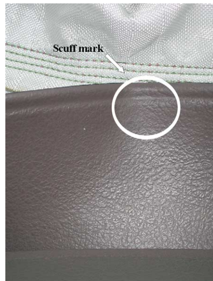
Figure 31 Nonpatterned scuffmark on module cover from hand placement. Injuries of each occupant can be matched to module cover damage.
