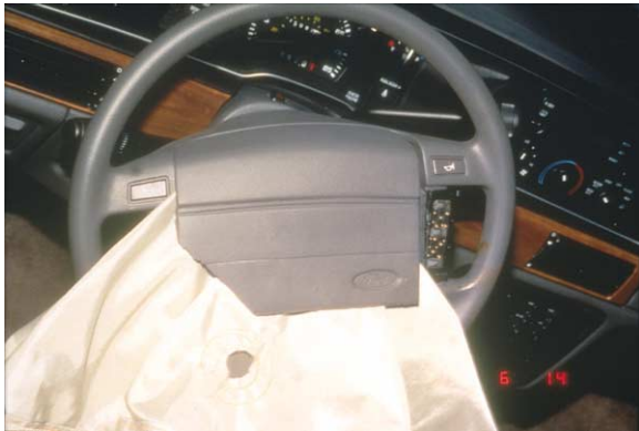
Figure 2 The canvas airbag and the module cover are both capable of inflicting serious and fatal injuries. Reproduced with permission Smock WS. Accident Investigation: Airbag-related Injuries and Deaths. In: Encyclopedia of Forensic Sciences . Edited by Jan A Siegel, Pekka J Saukko, Geoffery C Knuufer. Academic Press: London. © 2000 with permission from Elsevier.
