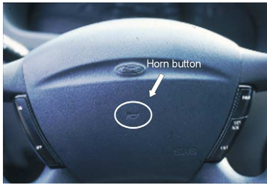
Figure 4 Air bag module covers with built-in horn activation buttons are an invitation for serious injuries to the upper extremity (Figures 5, 21–28).
