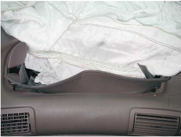
Figure 29 Deformation of the passenger module cover from arm placement (Figure 30).
